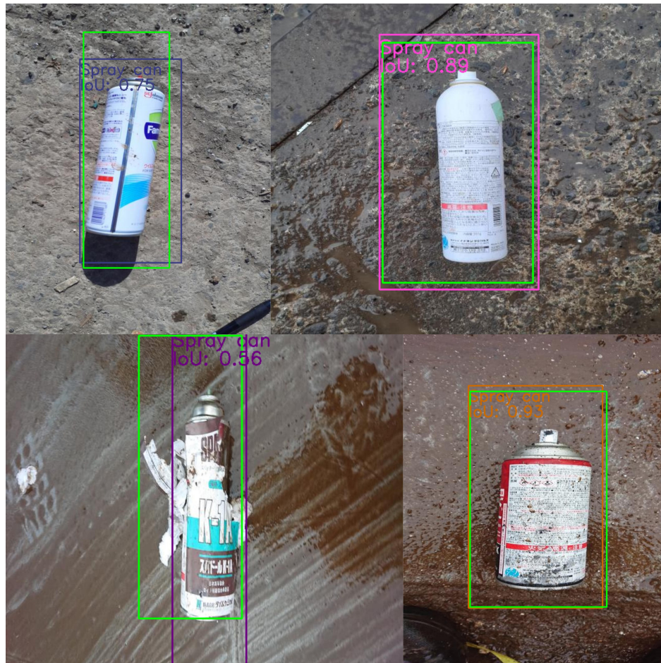
Figure 6: This figure represents the detailed IoU evaluation for detected spray cans, showcasing the model's ability to accurately delineate the contours of this specific hazardous object. Each spray can in the image is associated with an IoU value, affirming the model's precision and reliability in real-world implementations
