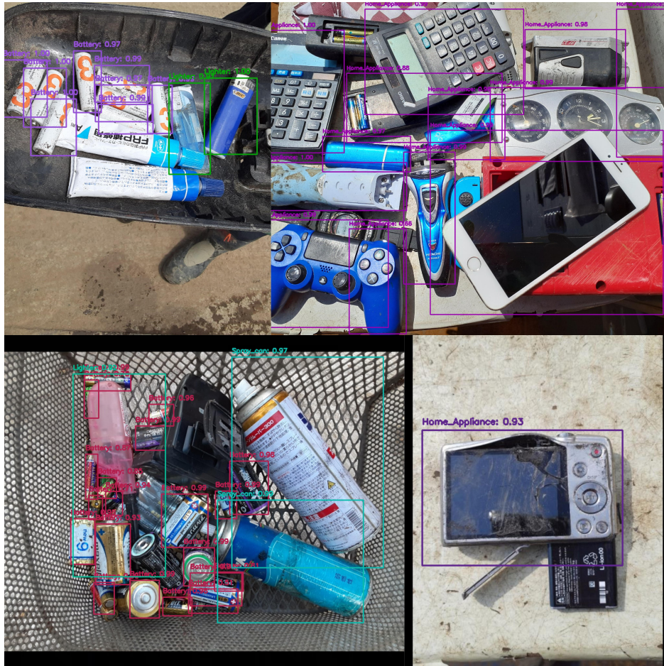
Figure 4: High confidence detection of recycle plant hazardous items
